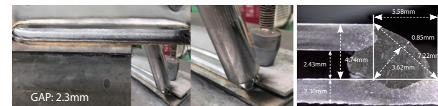
[ 590MPa Zinc Coating Steel 2.3mmt LAP JOINT, Ar+CO 2 (9:1), 180A/16V ]
